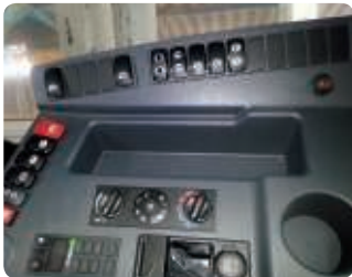
Centralized Instrument switch Panel
