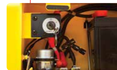
Master Switch A master switch disconnects the battery power to protect the electrical system from excess electrical drainage.
