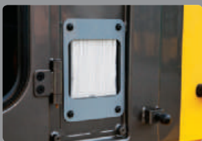
Cabin air fresh filter The pressure inside the cabin is slightly higher than outside. This excludes dust from the cabin and reduces noise levels.
