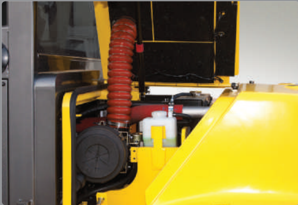
Dual element air cleaner (8") The air filter is readily accessible for cleaning or replacement. The large size of air cleaner extend the life time of engine.
