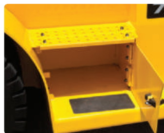
Large tool box Additional tool box located under footstep for operator's convenience.
