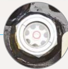
Hydraulic Oil Level Gauge
